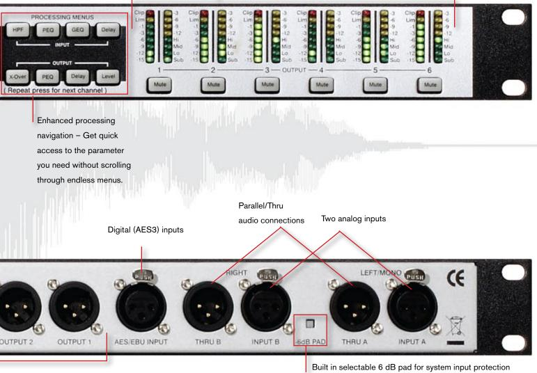
Built in selectable 6 dB pad for system input protection – this analog pad is placed before the A/D converter to provide extra protection against input clipping caused by devices with high output levels, such as DJ mixers.
