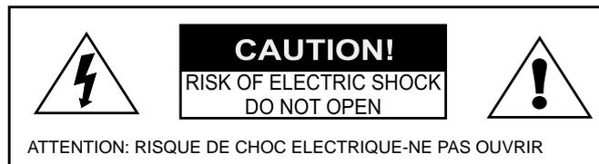
19. The lightning flash with arrowhead symbol within an equilateral triangle is intended to alert the user to the presence of non-insulated "dangerous voltage" within the product's enclosure that may be of sufficient magnitude to constitute a risk of electric shock.
